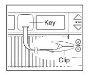
the displays will light. IMPORTANT: In an emergency, the key can be pulled from the console, causing the walking belt to slow to a stop. Test the clip by carefully taking a few steps backward; if the key is not pulled from the console, adjust the position of the clip.
